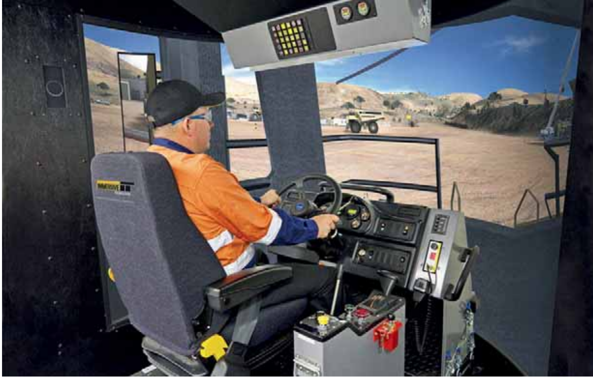
The surface mine vehicle simulators dynamically adjusts viewing perspective to offer a real world view from the cabin.
