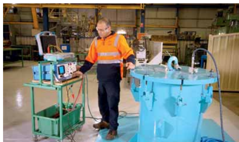
A purpose built pressure Test Emersion Tank to simulate bore conditions.
