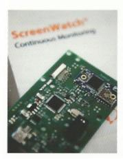
A new smart monitoring system that helps our customers better understand the condition of their vibrating screens recently made its Australian debut.
