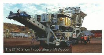
A significant achievement was the recent supply and commissioning of a new LT140 mobile crushing unit, which is part of BGC's processing system that is handling the contract crushing at Mt Webber.
